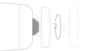
Each attachment can be easily and effortlessly attached or removed by twisting it 90°.
